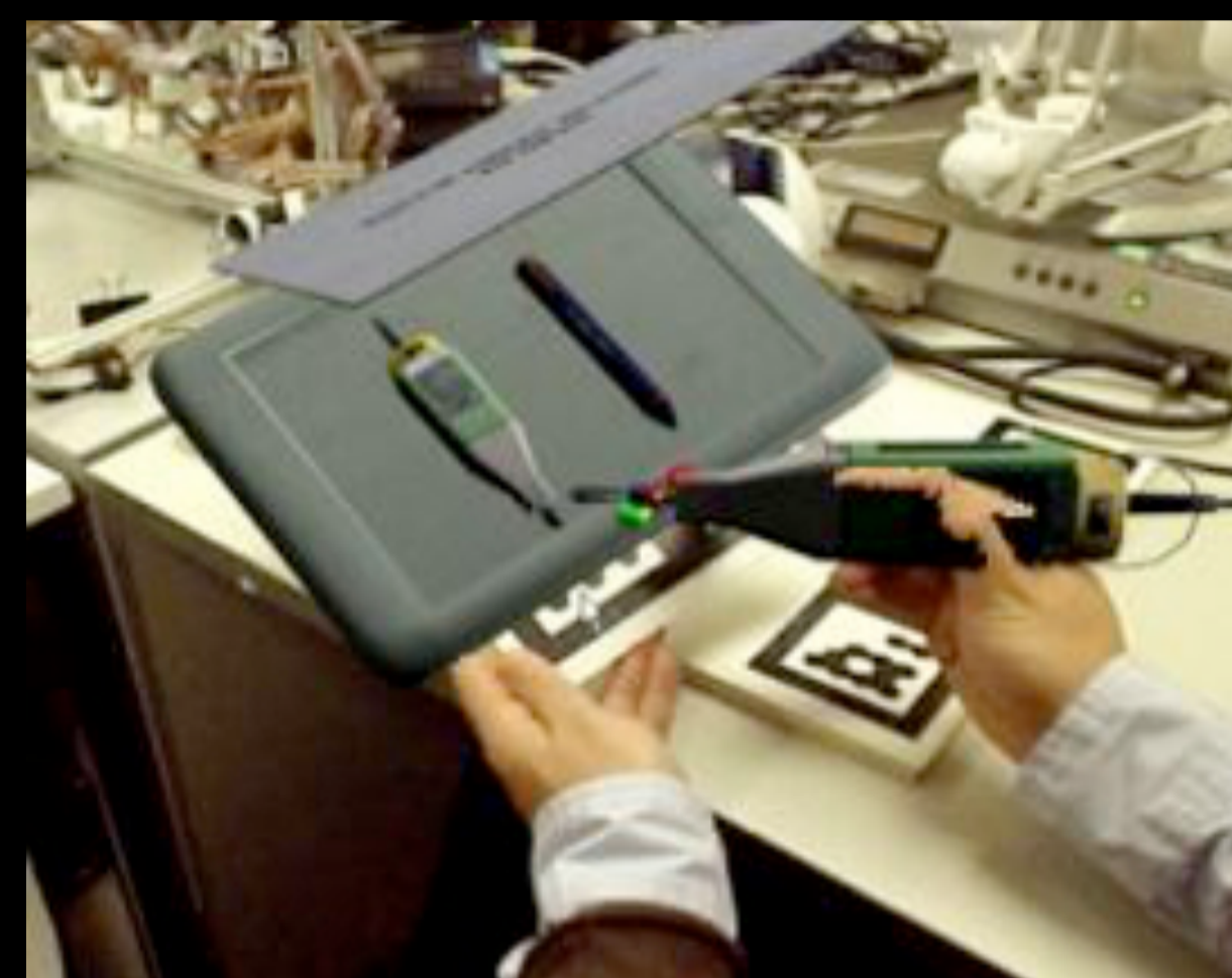
Virtual tools are overlaid onto the haptic device
