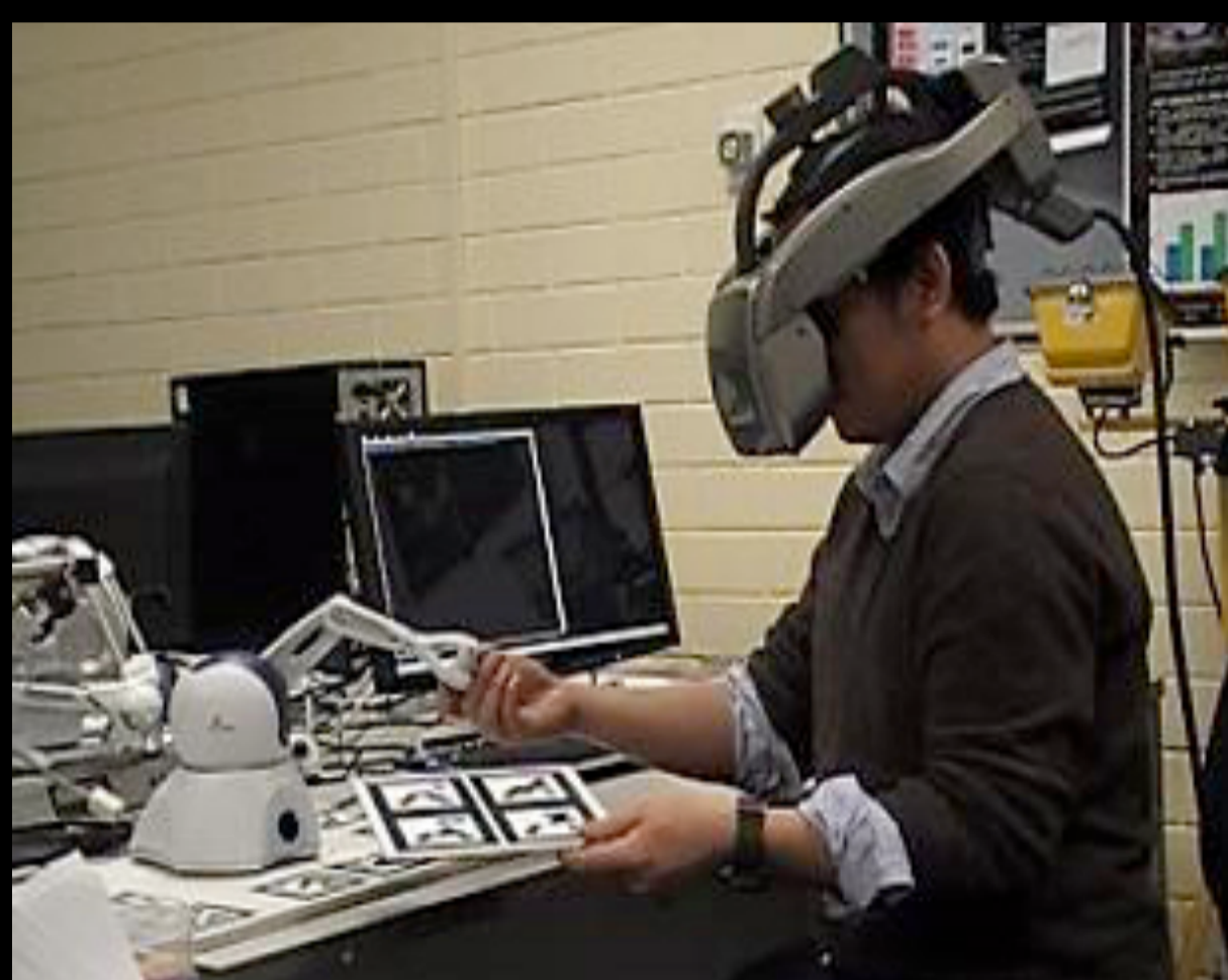
VHAR setup with a head-worn display and a haptic device
