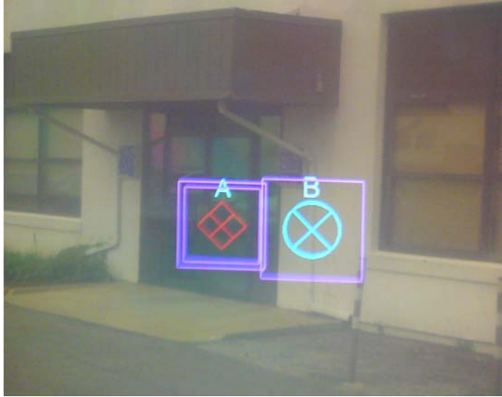
Fig. 11 This customized and simplified version of the virtual tunnel concentrated on the number of planes through which the tunnel was being extended to get to the target object. It was the best method in a broad-based comparison of X-ray vision metaphors [28].
