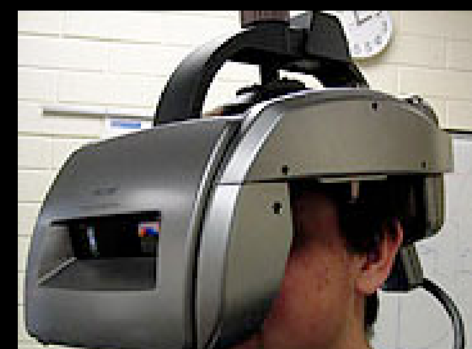
Canon COASTAR-type head worn display VH-2007 with wide field of view (60 degrees horizontal).
